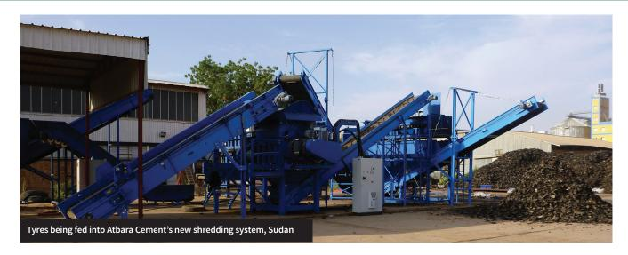
A tbara Cement Co recently added a shredding line at its plant situated in Atbara, northeastern Sudan, to prepare waste tyres for use as an alternative fuel. Supplied and assembled by Terier sro, the line processes tyre chips to dimensions of 50-100 x 50-100mm. It has a throughput of 2-5tph and is equipped with a tyre shredder, radial mesh screen and four conveyors.
